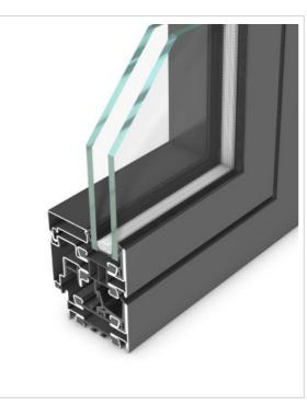
Bullet-resistant, non-insulated system in compliance with resistance classes FB4 and FB6 (with armouring/panelling) for doors and partition walls made of steel
